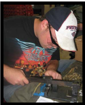
Brandon removing bushings using a jig within our manufacturing area, notice he is following proper safety procedures and wearing safety goggles.
